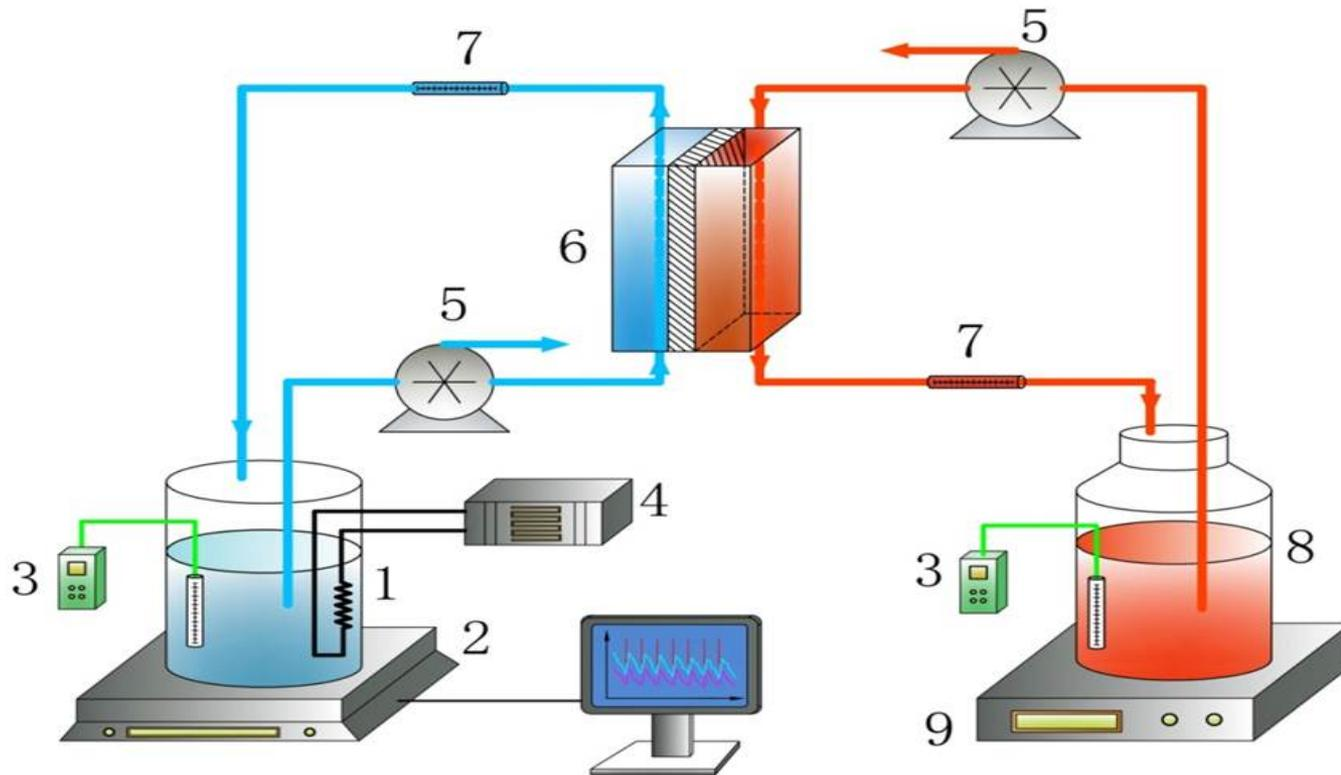
**Figure 2.** Schematic diagram of the DCMD test unit (1: Permeate tank, 2: Digital balance connected to a computer, 3: Thermometers, 4: Cooling unit, 5: Pumps, 6: Flat sheet membrane module, 7: Flow meters, 8: Feed reservoir, 9: Hotplate).
