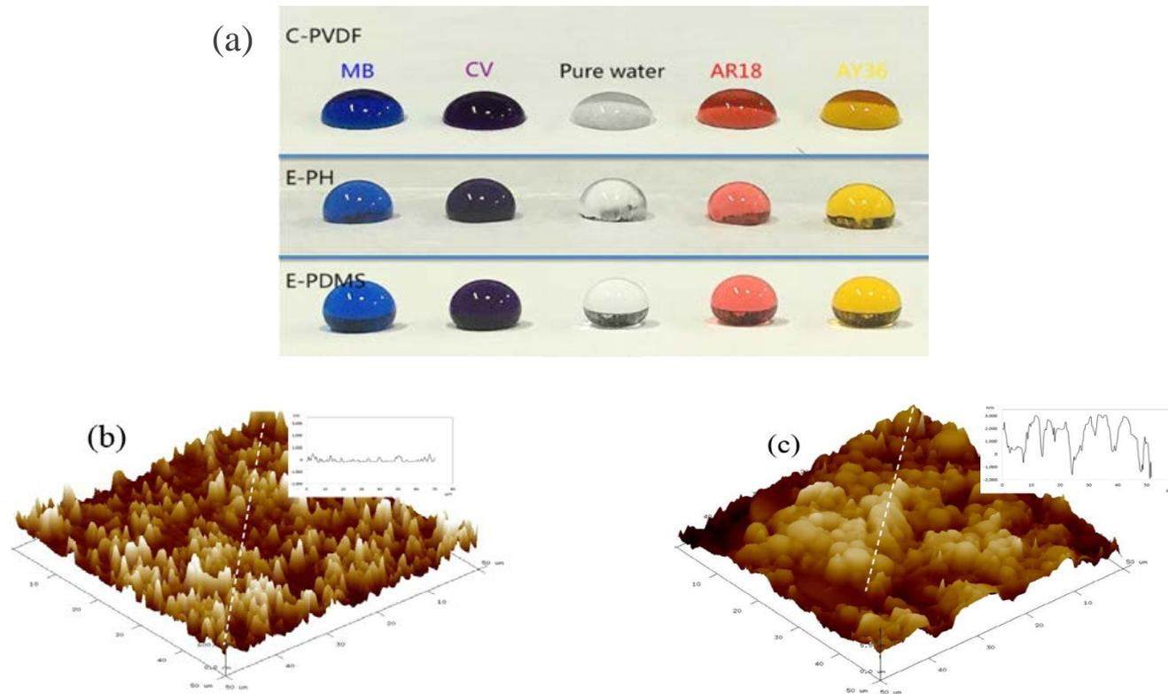
**Figure 5.** (a) Pure water and dye droplets on the surfaces of the three different membranes (C-PVDF, E-PH and E-PDMS) and (b) C-PVDF and (c) E-PDMS membranes' roughness analyzed using AFM.
