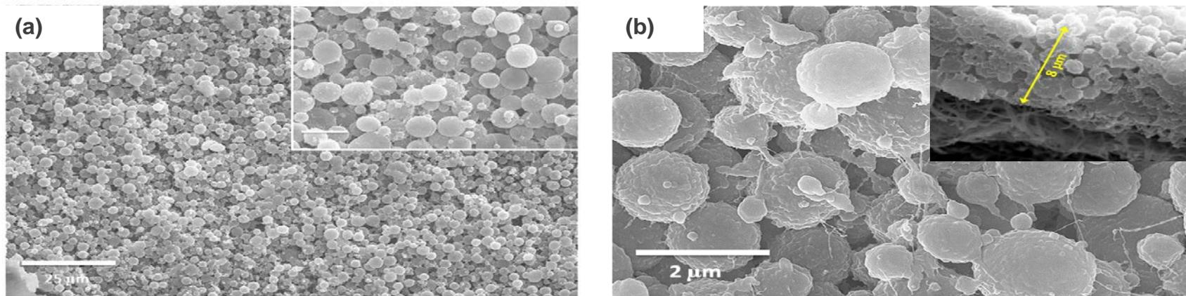
**Figure 3.** SEM images of the of E-PDMS membrane laboratory-fabricated (top right of b: cross-sectional SEM image).
