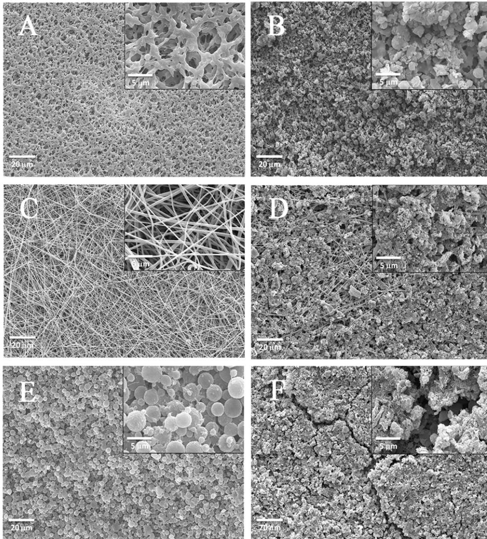
**Figure. 9** SEM images (X2,000 and X15,000) of (a) the virgin C-PVDF membrane, (b) the C-PVDF membrane after MD, (c) the virgin E-PH membrane, (d) the E-PH membrane after MD, (e) the virgin E-PDMS membrane, and (f) the E-PDMS membrane after MD in CV treatment.
