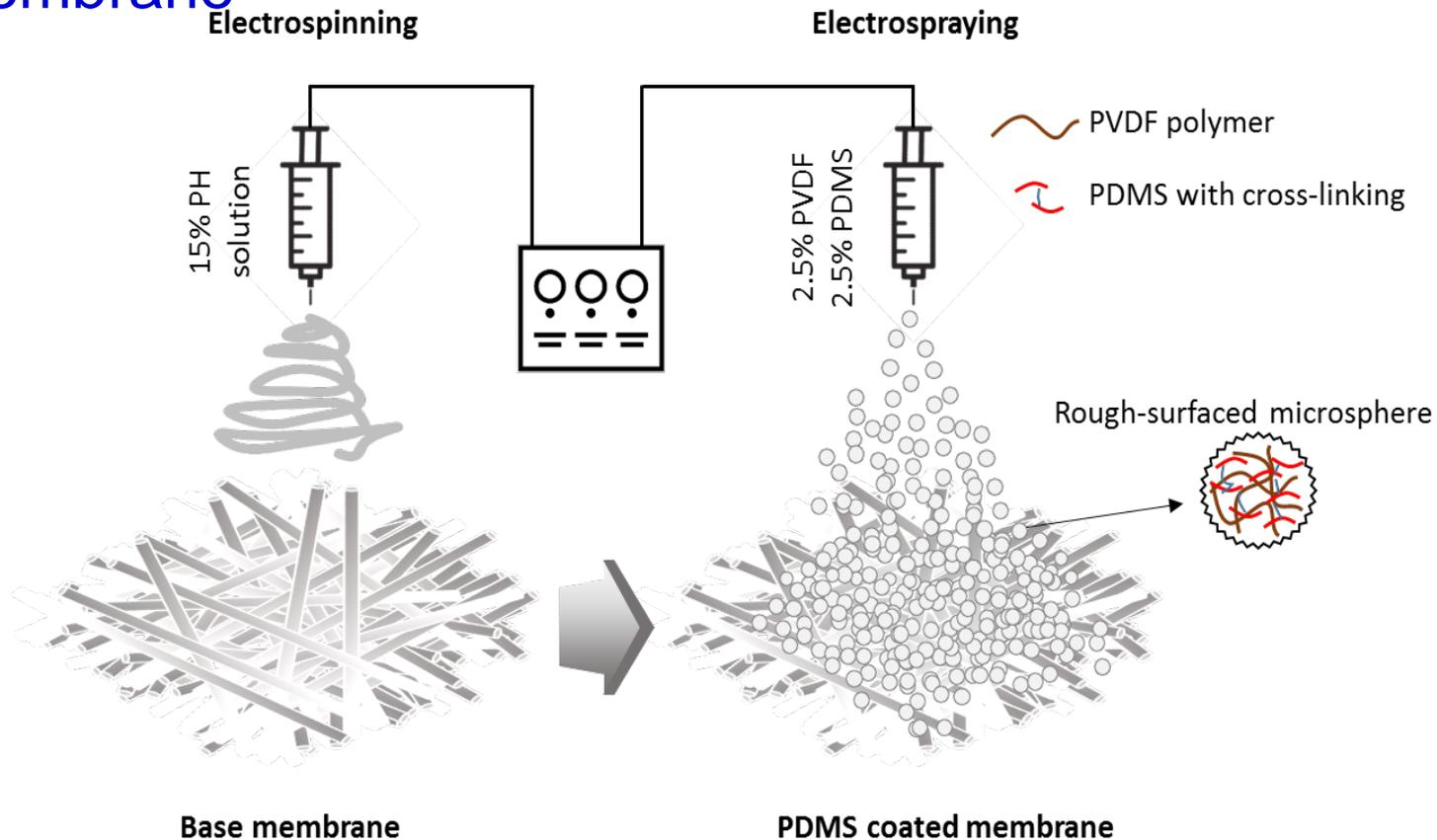
**Figure 1.** Schematic illustration of hybrid PDMS/PH membrane (E-PDMS) fabrication.
