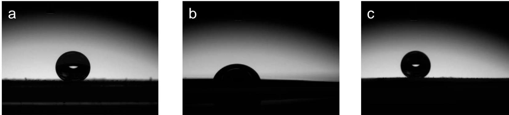
**Figure 11.** Behavior of a water droplet on the surface of the E-PDMS membrane (a) virgin membrane, (b) after 24 h of MD operation, at which point the CA dropped from 155.4 to 87.1°, and (c) after WF for 10 min, in this case the CA was 99% recovered to 154.9°.
