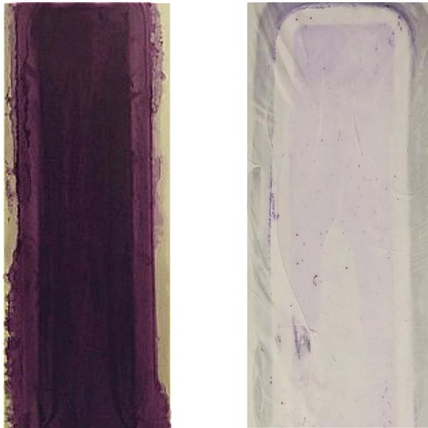
**Figure 12.** The surface picture of (a) C-PVDF and (b) E-PDMS membranes after 24 h MD operation with WF for CV treatment.
